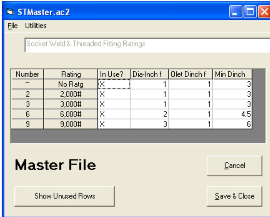
Note that ST3 is applied only to olet welds with an associated fitting rating. It enters the calculation BEFORE the on-fitting factor (OF) and BEFORE the material group factor, MG1.
